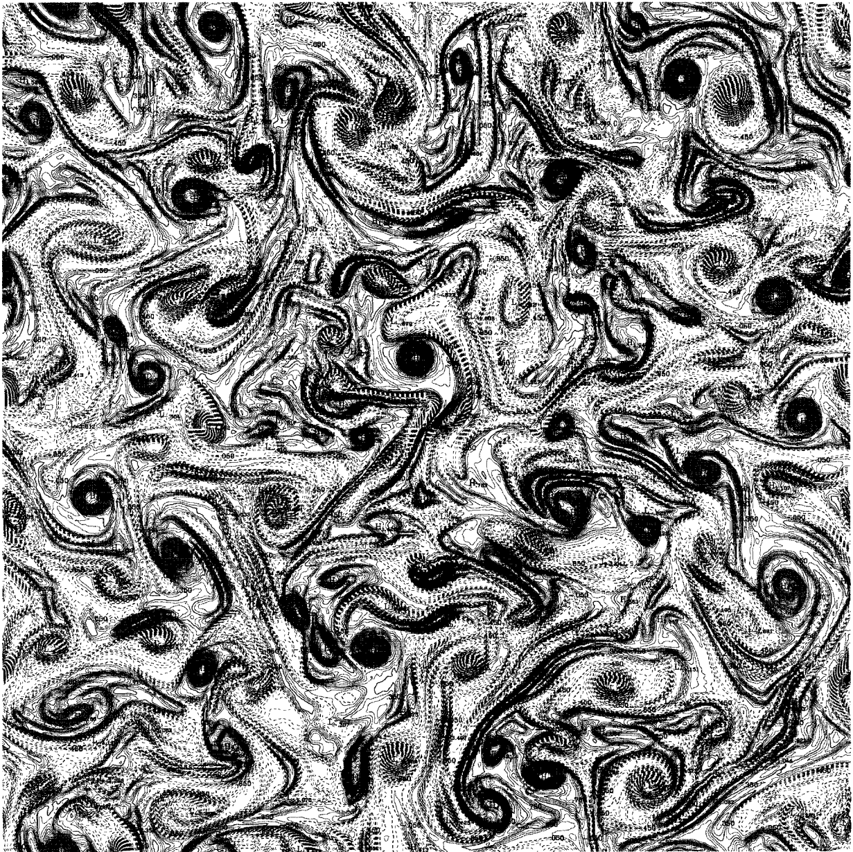
FIG. 8a. Snapshot of vorticity field at t \approx 25.9 for turbulent flow simulation computed with sixth-order accurate advection scheme with ELAD. Grid resolution is 256 \times 256 . The whole computational domain is shown. Minimum and maximum values are \pm 10 , contour interval is 0.1, so that there are approximately 200 contour levels on this plot. Negative values are contoured in dashed lines.
